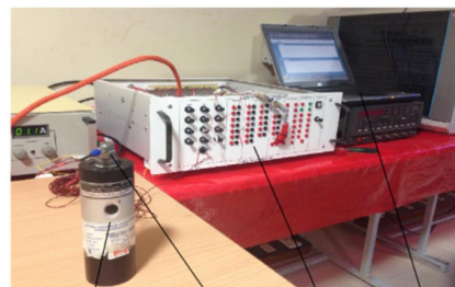
Figure 9: Accelerometer calibration set-up.
