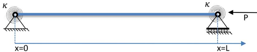
Fig. 5. A generally constrained beam subjected to axial force
