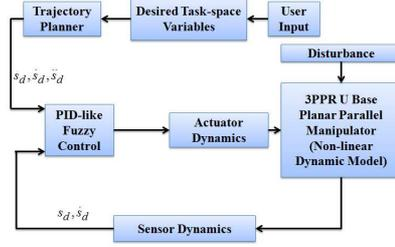
Figure 4: Linear PID-like fuzzy controller block diagram
