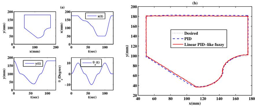
Figure 5: (a) Task-space trajectory (b) Task-space trajectories of the end-effector during complex trajectory tracking
