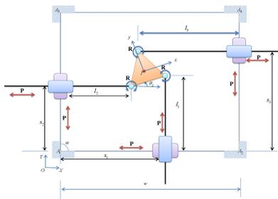
Figure 1: Frame diagram of the 3PPR U-base PPM
