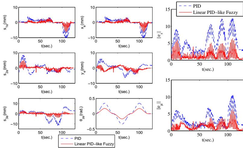
Figure 6: Linear time trajectories of the joint-space and task-space position tracking errors
