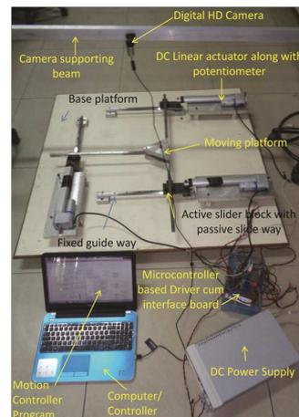
Figure 2: Experimental setup of the 3PPR U-base PPM
