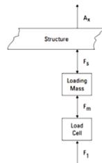
Fig. 7. MASS LOADING OF SHAKER
