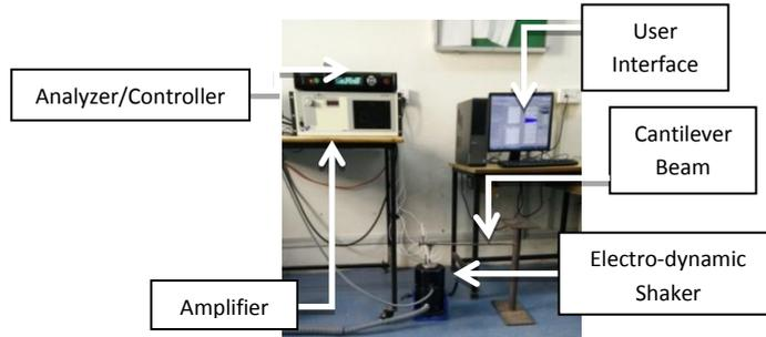
Fig. 6. SHAKER TEST SETUP
