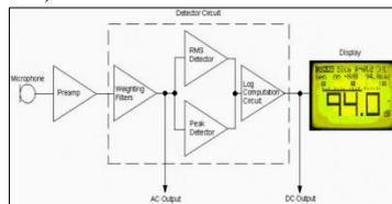
Fig. 10. FUNCTIONAL DRAWING OF SLM
