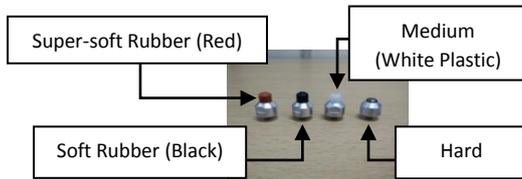
Fig. 2. DIFFERENT IMPACT HAMMER TIPS
