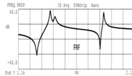
Fig. 9. SHAKER/STRUCTURE IMPEDENCE MISMATCH
