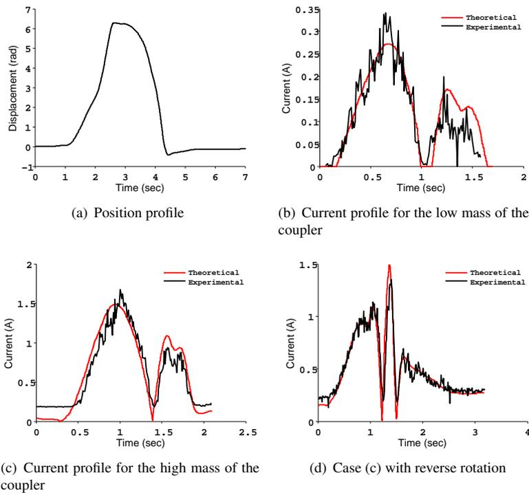
Figure 3: Experimental outcomes for the crank-rocker four-bar mechanism
