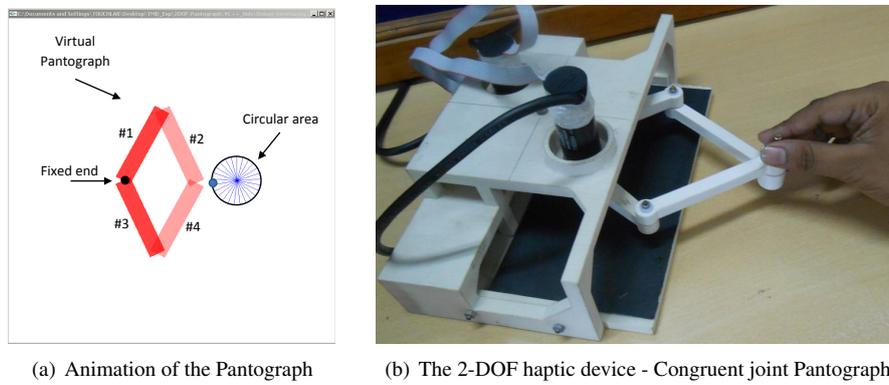
Figure 4: Two-DOF mechanism dynamics simulation
