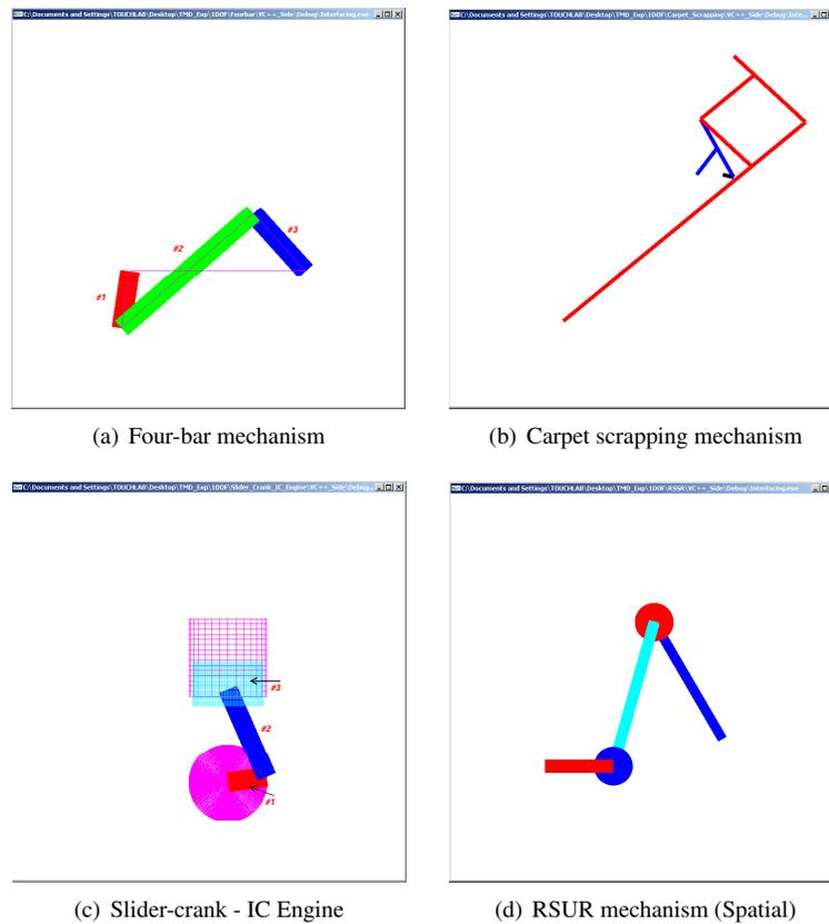
Figure 2: Animation windows of one-DOF mechanisms
