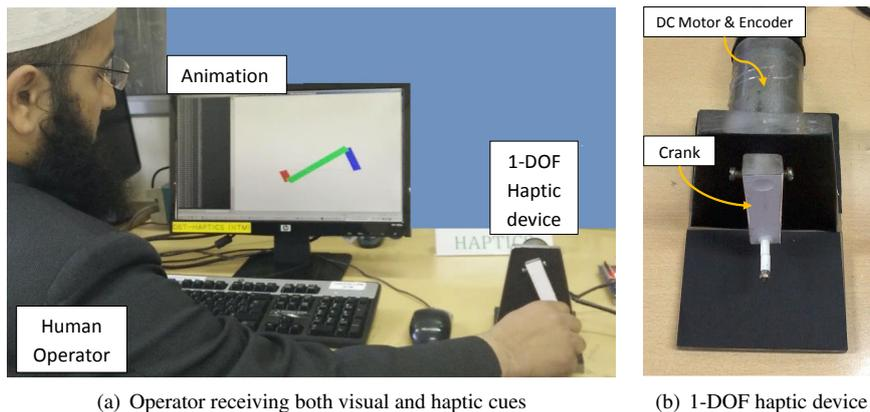
Figure 1: A typical teaching mechanism dynamics setup
