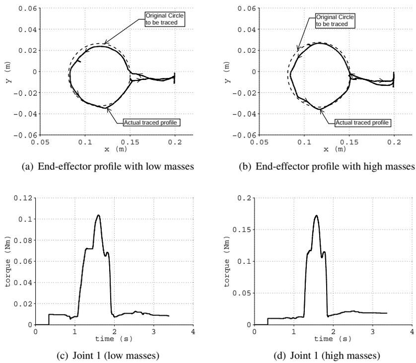
Figure 5: End-effector and active joint torque profiles for drawing circle with the 2-DOF haptic device
