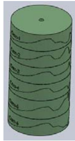
Figure 5a: Common Cam Six Leg Profiles
