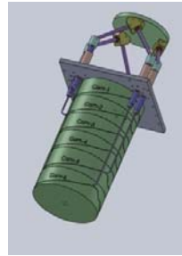
Figure 5b: 6-PSS based Common Cam Manipulator
