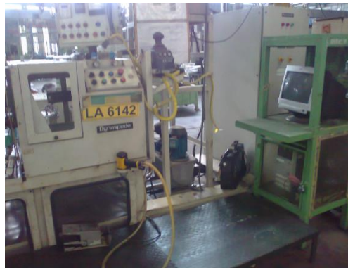
Figure 5: AMT gearbox test rig with prognostic observer inbuilt controller.
