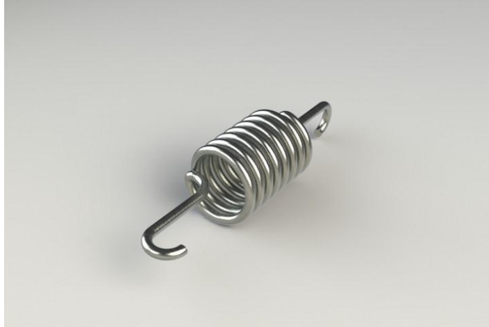
Figure 2: SOLIDWORKS model of nitinol spring
