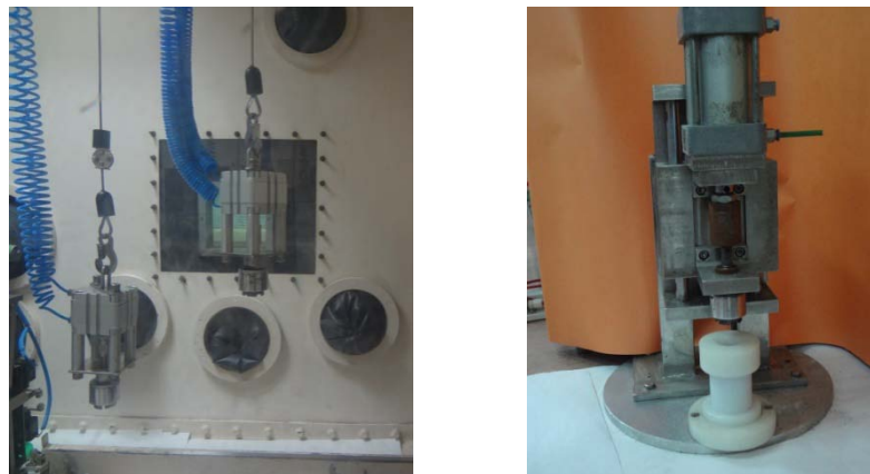
Figure 8: Hanging type sealing and unsealing tool powered by the pneumatic actuator installed inside the STB and a unsealing machine installed on the STB floor
