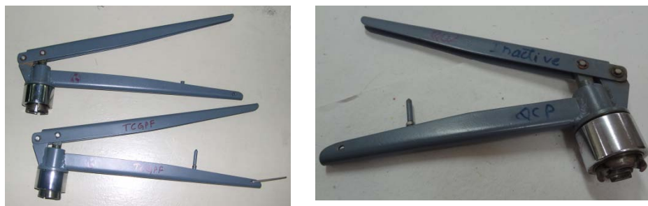
Figure 3: Vial Sealing tool, vial unsealing tool
