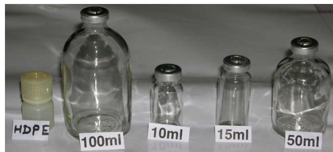
Figure 2: Crimp top glass vials used for storage and transport of the RPhs
