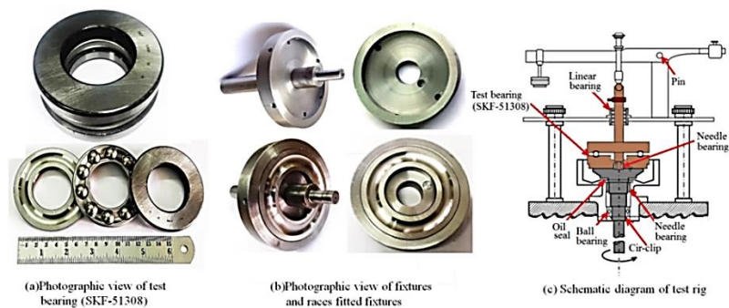
Fig.1 Photographic view of test bearing (SKF- 51308) and schematic representation of bearing mounting and loading on the test rig
