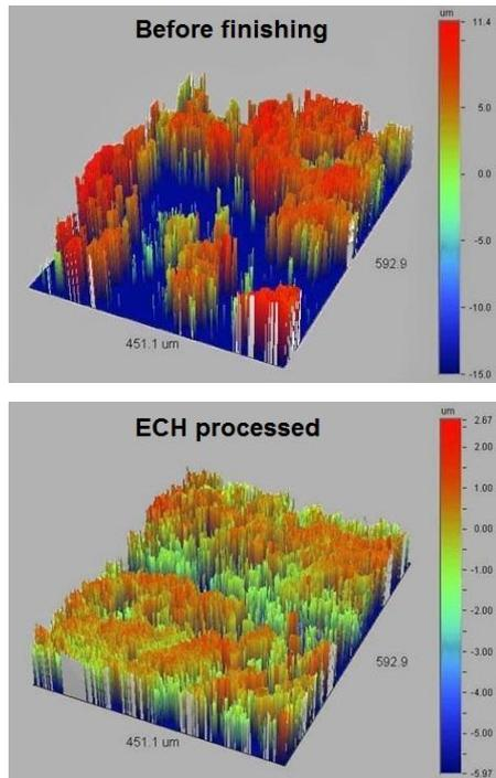
Figure 4: Topography of the workpiece surfaces obtained through optical profilometer
