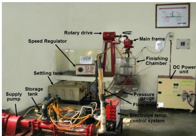
Figure 2: Photographic view of the developed ECH setup
