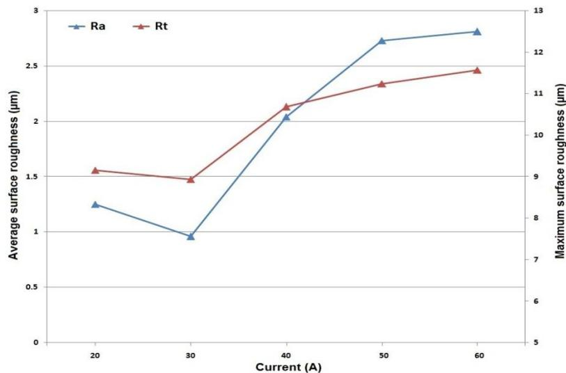
Figure 3: Plot Ra/Rt - current
