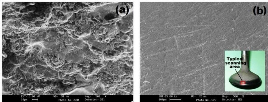
Figure 5: Typical SEM micrographs (a) prefinished; (b) after ECH
