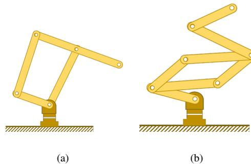
Figure 1: Target basic morphologies: (a) Five-bar chain mechanism with two degrees of freedom, (b) Close loop within serial chain
