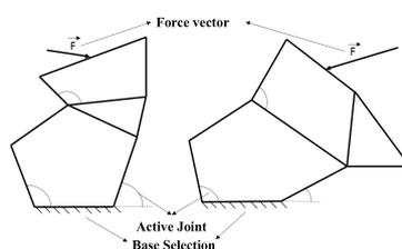
Figure 2: Selection of base, active joints, and point of application of force
