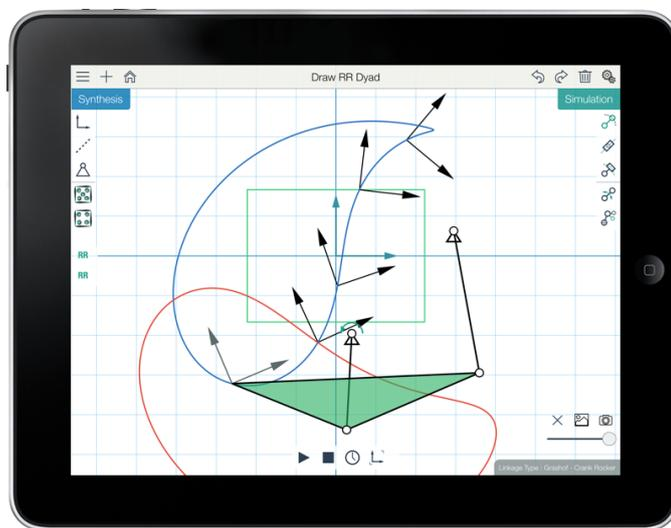
Figure 3: A planar four-bar linkage synthesized for a sit-to-stand motion; the *blue* curve shows the path of the hip joint being traced by the coupler point; the *red*-curve shows the other circuit.
