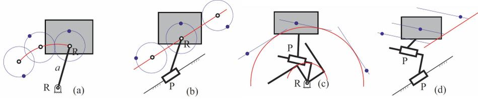
Figure 2: Planar dyads: RR, PR, RP, and PP
