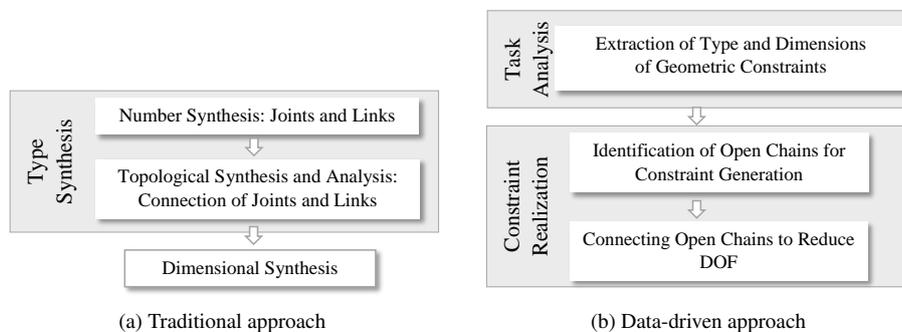
Figure 1: Traditional approach vs Data-driven approach: In the Data-driven approach, the first step is to extract the geometric constraints implicit in a given motion, and then to match them with appropriate mechanical dyads before connecting two of them to form a single-DOF mechanism.
