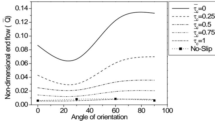
Fig.4 Effect of texture orientation on load support for different critical threshold shear stress values
