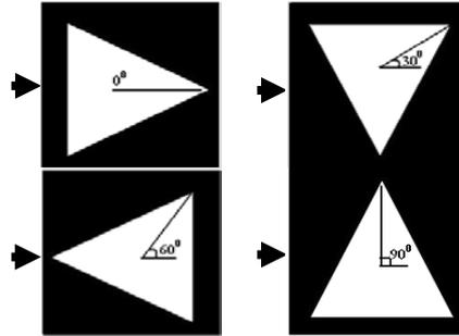
Fig.1 Orientation angles of triangular texture. Arrow mark indicates the fluid flow direction
