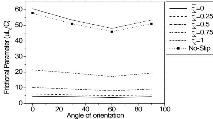
Fig. 5 Effect of texture orientation on friction parameter for different critical threshold shear stress values
