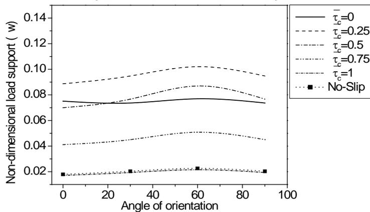
Fig. 3 Effect of texture orientation on load support for different critical threshold shear stress values
