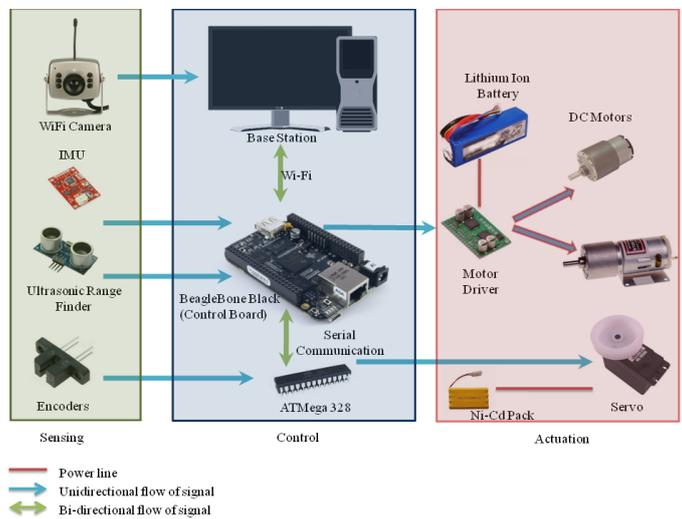
Figure 6: System architecture
