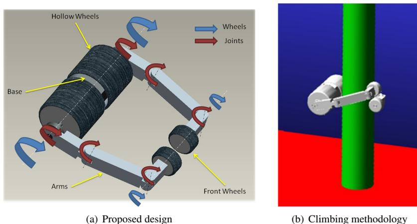
Figure 1: Inspection robot
